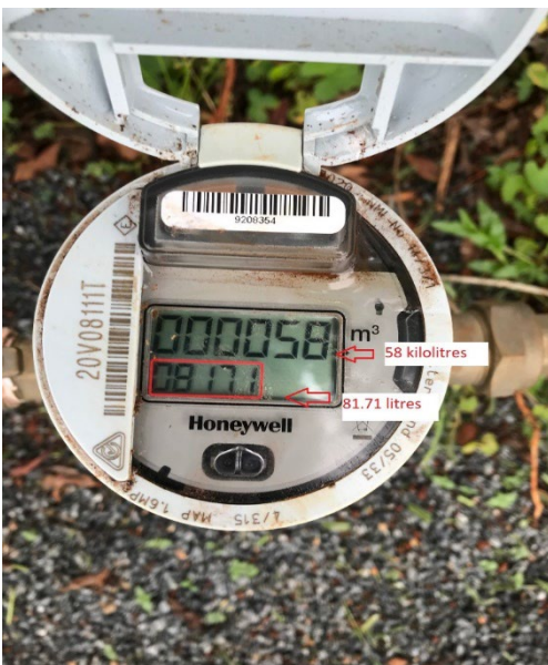
Photo Left: V200 –HT showing 58 kilolitres and 81.71 litres (ie 58.08171 KL)
