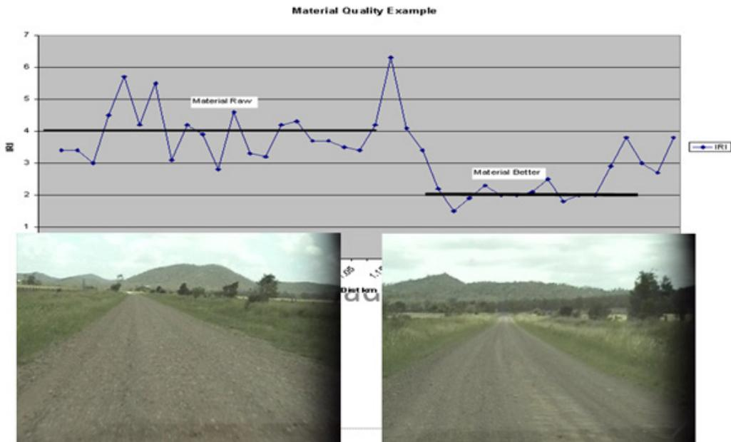
Figure 2.2d: IRI Chart Illustrating Effect of Material Quality on Road Deterioration
