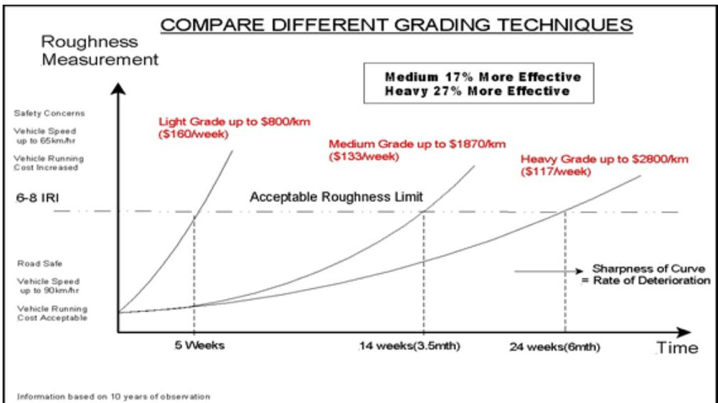
Figure 2.1c: Comparison of Grading Techniques Over Time
