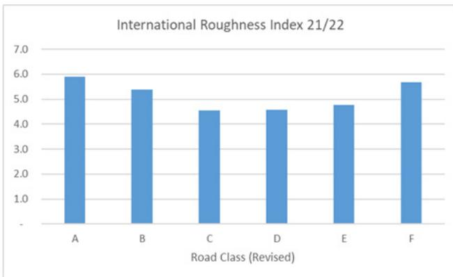
**Figure 3.3.1d: International Roughness Index Results for CCRC Road Network**
