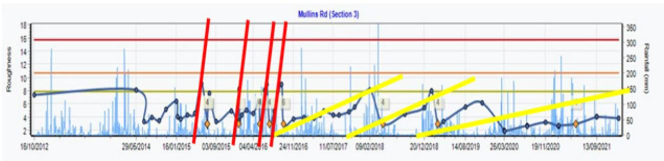
**Figure 3.3.1a: Deterioration charts of medium grading and heavy grades**
