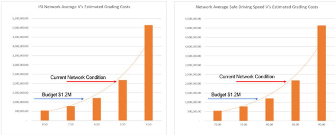
**Figure 3.3.6a: IRI vs Estimated Grading Costs and Safe Driving Speed vs Estimated Grading Cost**
