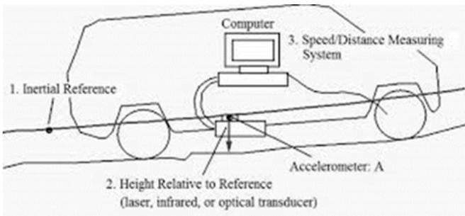
Figure 3.3.1a: How International Roughness Index (IRI) is Measured
